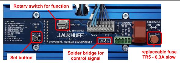
The S.1 magnet sets the benchmark for the most advanced generation of slider solenoids. It uses four optical sensors for measuring the motion speed of the slider. The automatic force adjustment feature sets the perfect speed assuring that the magnet comes to a soft and silent stop at the end position. The control circuitry readjusts the force in case of load changes so that the slider moves at optimum speed and reaches the exact end position without fail.
