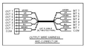
An output wiring harness, approximately ten feet in length, comes with the UAE128P. The end that plugs into the board is pre-terminated with an 8-pin connector while the other end fans out for connection directly to shade operator or to an organ control system.
