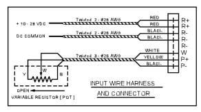
An input wiring harness, approximately three feet in length, comes with the UAE128P. The end that plugs into the board is pre-terminated with an 8-pin connector while the other end fans out for connections to the console power supply and the POT. It is recommended that the board be located as close to the POT as
